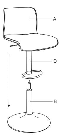
Step 4. Pull up lever on footrest (part D) to adjust the seat to suitable height.
